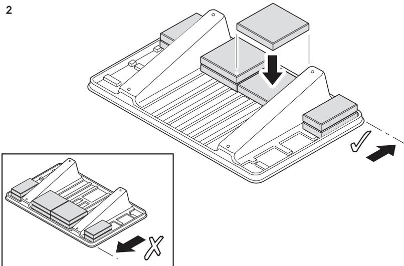
EN **Note:** The tiles should be placed at the back of the bottom plate as much as possible.
